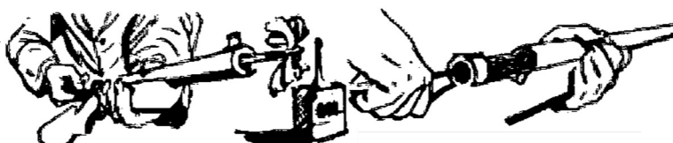
Run oily patch through barrel
