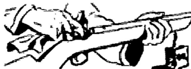
All metal parts should get light coat of oil
