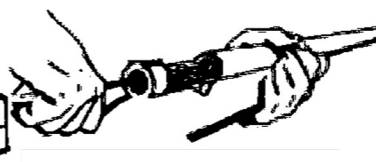
Bore should be cleaned through breech end when possible
